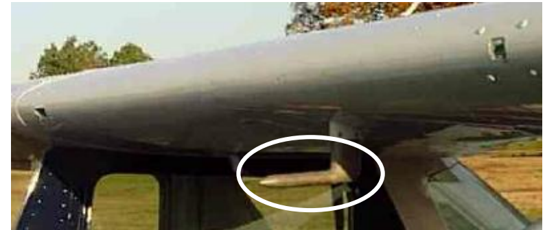
Pitot tube mounted on airplane
